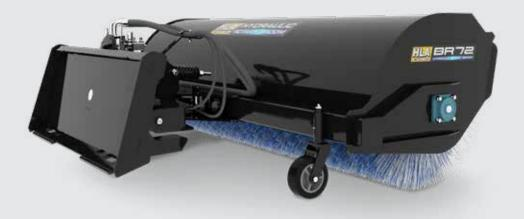
The hydraulic rotary broom comes ready with everything you need including hydraulic hoses, flat-faced couplers, and an electric selector valve, and wire kit. Hooked up and ready to go, the broom's direct motor drive requires 12-20 GPM of hydraulic flow to turn the 26" diameter poly/steel wafers.
