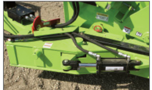
Optional hydraulic swing hitch
