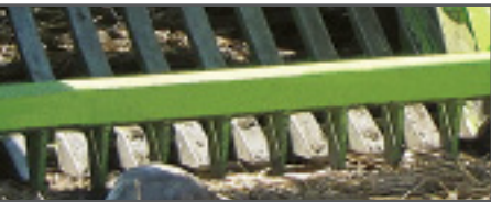
Wide grate for minimum till picking
