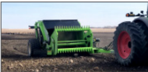
Wide grate for minimum till picking
