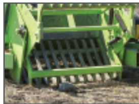
Minimum till wide grate & reel 3 9/32" spacing
