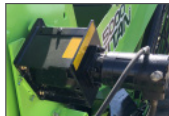
The direct drive motor has a built in cushion valve No chain or sprockets used
