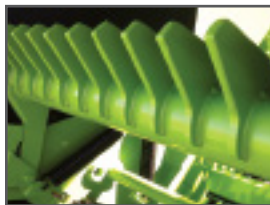
Heavy duty grate & reel 450BNH 1/2" spacing & replaceable teeth
