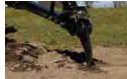
Ripper Tooth for breaking hard ground available on GX720, GX920, GX920XT
