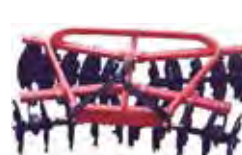
3 point disc harrows 4' 4" to 11' 4" working widths.
