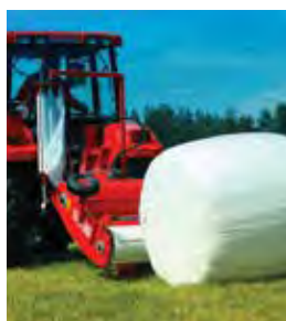
Bale is unloaded by raising the table with the 3 point lift.
