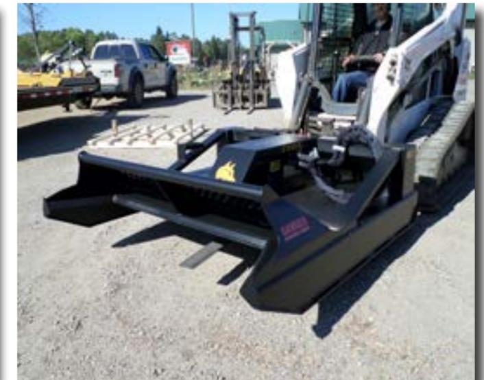
Open front cutters have become increasingly popular for their ability to selectively cut vegetation with the use of exposed blades. The 7201 line up of brush cutters come with all the quality driven features found on our heavy duty models along with incorporating the "open front" concept. With exposed blades, this design is ideal for clearing grass, brush, and trees along buildings and fence lines.
