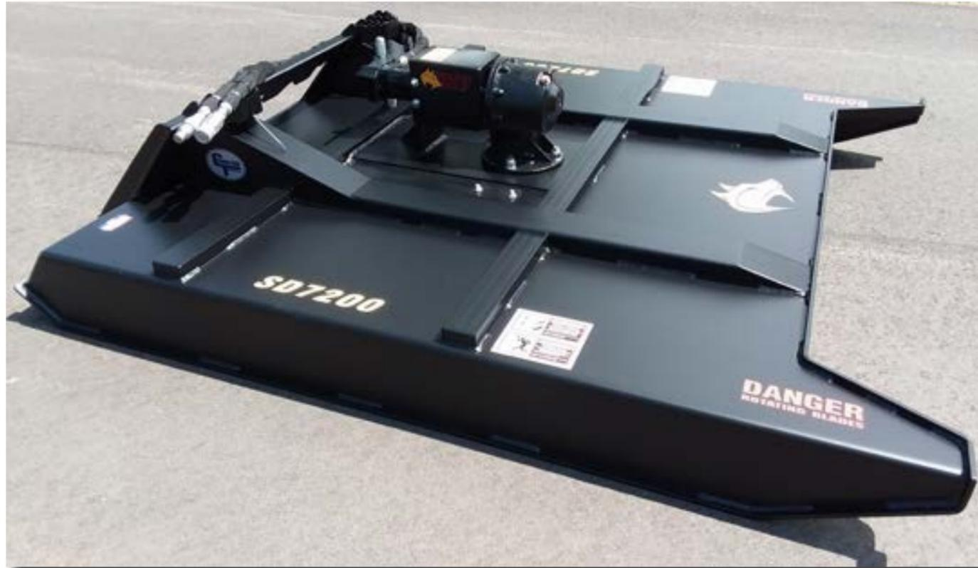
Standard duty models utilize all the same drive and blade carrier components as our tried and true heavy duty models at a more budget friendly cost. A lighter support structure, limited guarding, and removed chain curtains are some of the modifications made to provide a more economical cutter option.
