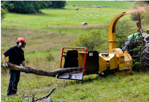
Hydraulic feed hoppers with a wrap-around lever that starts and stops the dual spring loaded rollers, maximizes chipping.
