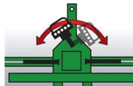
5 STICK CONTROL W/ SWIVEL Boom operational from either side of the trailer.
