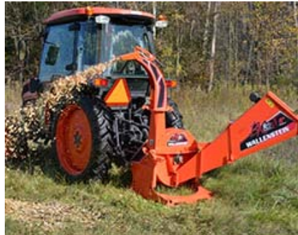
Self-feed intake hoppers are designed to angle the brush against the rotor and blades, pulling the branches into the chipper.
