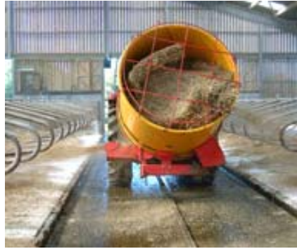
Discharging from both upper right hand and lower left hand chutes for free stall bedding. (standard on all C&B machines)
