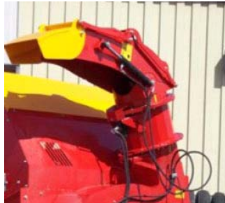
12" extension for T1010 chute to discharge to the rear of the machine
