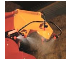
Hydro shield – dust suppression system
