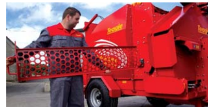
8555 CHIEF features 20% larger removable screen. The removable screens allow the 8555 to chop both wet and dry material.
