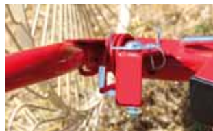
Rake Wheel Pressure Adjustment
