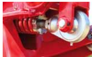
Hydraulic Cylinders to transition from working position to transport position
