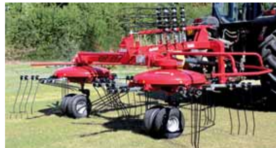
Single swath raking, working width 9' 10".
