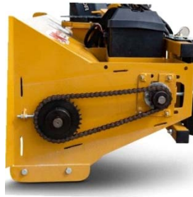
Roller chain connects the final drive between intermediate shaft and rotor
