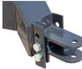
Adjustable Hitch ensures the mower is level
