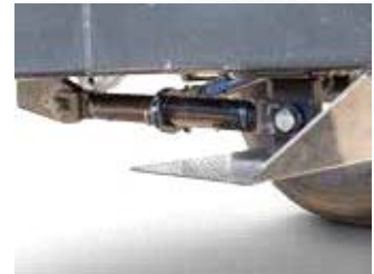
Hydraulic (option) lifts the mower up and down hydraulically
