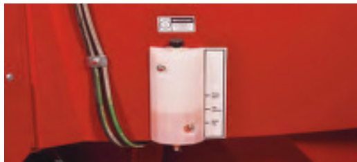
Oil Reservoir To monitor gearbox oil levels. Large & highly visible.
