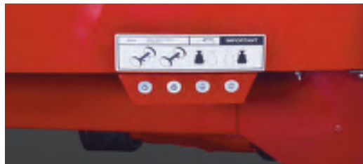
Central Grease Bank Regular maintenance is simplified as grease ports are routed to one bank. Standard on twin auger mixers.
