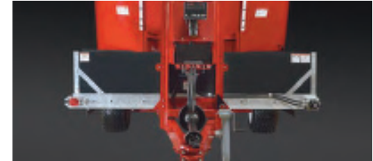
Dual Discharge Conveyor 8' or 9'2" Flat - not installed. Discharges feed to both the left & right side.
