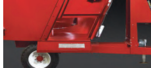
12" Chute Allows for easier placement of feed. Available with or without magnet.
