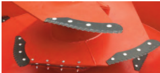
Tungsten Carbide Coated Knives Specially designed & oriented, ensuring max. cutting efficiency when processing long forage. Curved, carbide coated edges.
