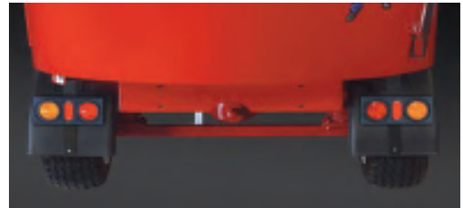
LED Light Bar Kit w/ Cable Indicator & warning lights for road travel. Flashing, warning, brake & turn signal.
