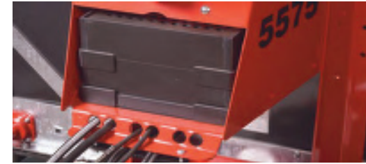
Shaker Box A simple way to test the uniformity of particle size & ingredient distribution in a batch and between loads to create an optimum mix.
