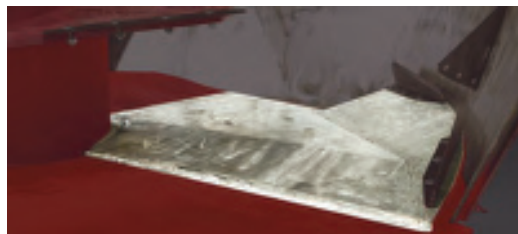
Stainless Auger Cladding The lead auger flights are coated in stainless steel to prolong the life of the auger.
