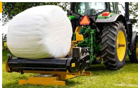
Manual Transport Lock: Secures bale platform to prevent dumping during transport.
