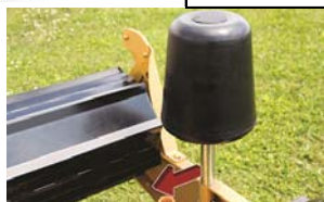
Adjustable Bale Guides: Allows 4' or 5' bales to be centered on the turntable.
