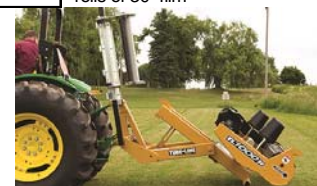
3 Point Hitch Lift: Easily unloads wrapped bales.
