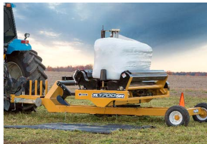
Drive Selection: allows the wrapper to switch between round and square bales
