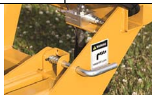
Manual Transport Lock: Secures bale platform to prevent dumping during transport.
