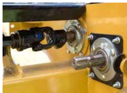
Drive Selection: allows the wrapper to switch between round and square bales
