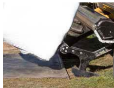
Bale Bumper: Ensures the bale lands far enough away from the table to rotate.
