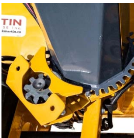
Electric chute rotator is standard and uses a wired remote to activate/rotate the chute
