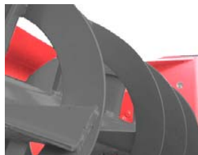
High Tensile Steel Ribbon Flighting
