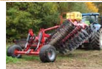
Seeder platform available for mounted/semi-mounted cultivator.
