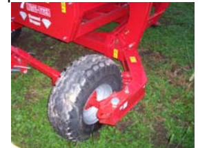
The right side wheel swivels out for more stability when wrapping, swings in for narrow transport.
