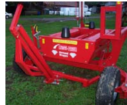
The right side wheel swivels out for more stability when wrapping, swings in for narrow transport.
