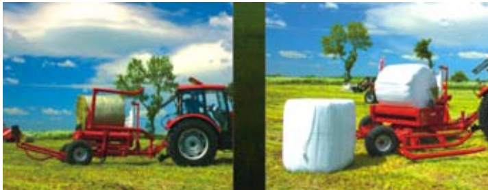
The right side wheel swivels out for more stability when wrapping, swings in for narrow transport.
