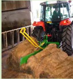
**MCHALE BALE SPLITTERS** are powered by one double acting hydraulic cylinder and a uniquely designed knife. The round bale splitter will securely transport the dry or silage bales from the stacking site to the feeding location. The operator simply splits the bale as desired in the feeding area or into a Feeder wagon. If the McHale round bale splitter splits the bale in the feed out area, it can also be used to push the bale segments into the feeding location.
