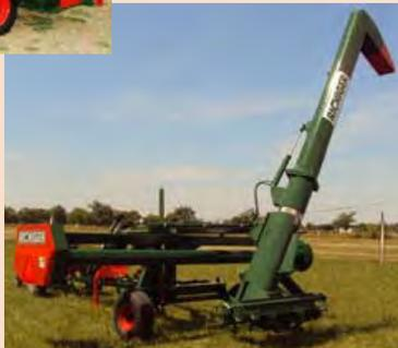
A 60 hp. tractor can unload dry corn at 300 tons/hr.
