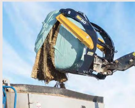
**BALE KNIFE** slices blades up to 72" in diameter. Top clamp grabs and retains plastic wrap and net wrap making it perfect for use with feed mixers.
