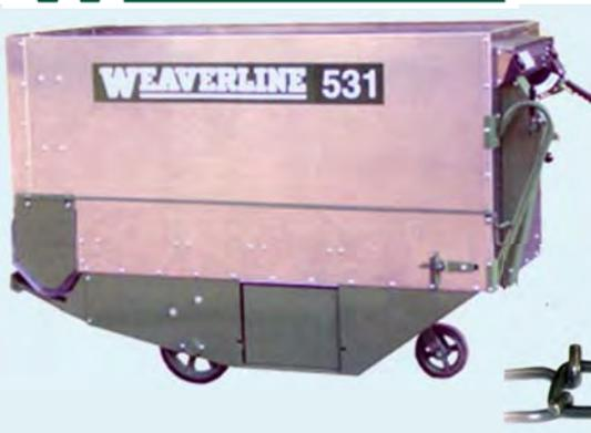
**WEAVERLINE ELECTRIC SILAGE CARTS** provide smooth efficient delivery of feed. Series 5 carts are designed for maximum durability and longevity utilizing stainless steel for all working components.
