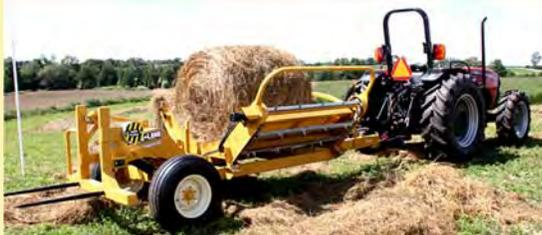
**BF5600 CHAIN TYPE BALE FEEDER** spears, lifts, separates, and serves hay straw or silage bales. All from the tractor seat. Spiked apron chain for positive rotation of bale. Fluffs hay as it's dispensed.
