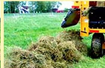
**TUBELINE'S BOSS II TRAILED SQUARE BALE PROCESSOR** is PTO driven and has a lift arm to load bales. Material can be broadcasted or windrowed.
