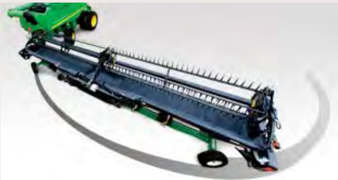
CHCF four wheel steer models for 30', 36' and 45' handle standard or draper headers.
