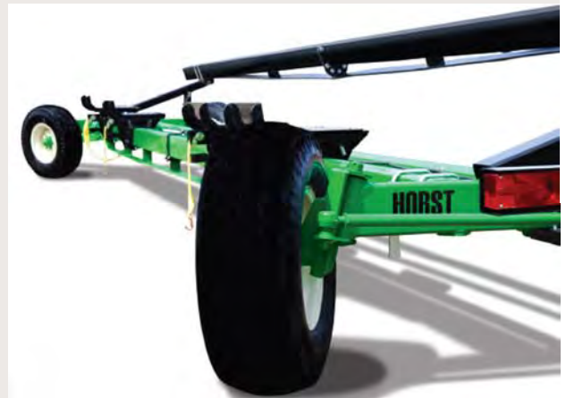
CHCF four wheel steer models for 30', 36' and 45' handle standard or draper headers.
