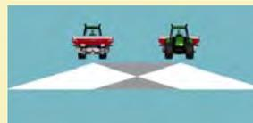
Double overlap spread pattern. Spread widths up to 148' with capacities up to 8200 lbs.
