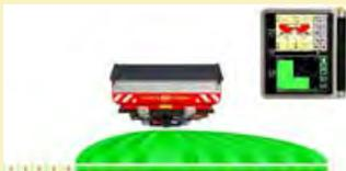
Decreasing the spreading width on the left hand side by 30'
