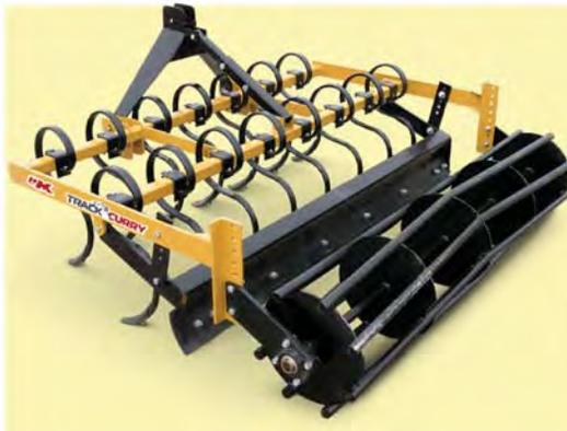
**TRACK CURRY**—This easy to use tool will allow you to condition the surface of your track to your desired firmness. With two rows of heavy duty S-tines to cultivate the ground, an adjustable leveling bar fastened to the rear of the S-tines and 12" rolling drum behind the leveling bar provides an accurate depth gauge to cultivate and pack your soil for optimum performance.
