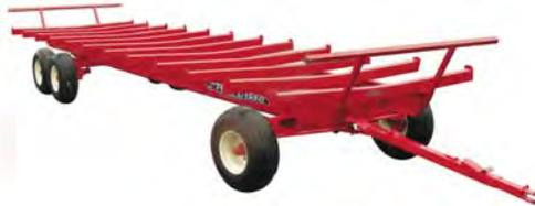
**ALL WELDED BALE RACKS** for 4' or 5' diameter bales. 20', 24', 30', and 36' lengths. 10" main beams (12" on 36') 5"x3" hss crossbars.
