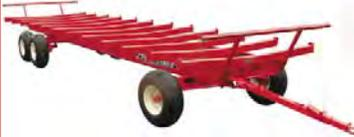
**MODULAR BALE RACKS** in 25', 30', and 36' lengths. Haul up to 34 bales on a 36' unit.
