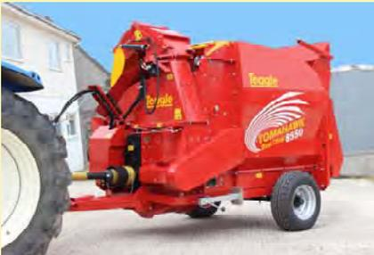
"Dual Chop" models have the ability to produce long chop or short chop material for slotted floors and liquid manure systems.
