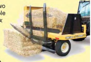
**BOSS IV** provides increased capacity by up to four 4'x4'x9' bales. Bales are easily loaded with the hydraulic self loading deck. Raise the deck to spear your stack then lower it back into position.
