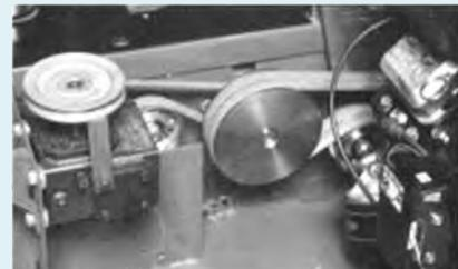
Double V belt drive system for efficient power transfer. Enclosed oil bath gearbox.
