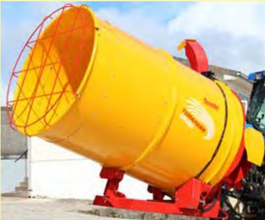
**MODELS T5050XL AND T505XLM** are equipped with a 9' long drum capable of handling full size square bales.
