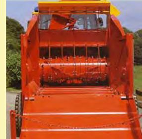
**TOMAHAWK SERIES** machines handle full size square bales and up to two 5' round bale. High volume model 1010 handles up to two full size square bales and three 6' diameter round bales. The swivel chute rotates 280 degrees so material can be directed wherever it's needed.
