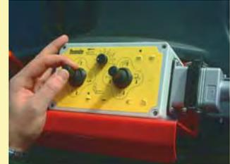
Electric over hydraulic controls for apron chain, chute rotation/up and down, and rear loading gate.
