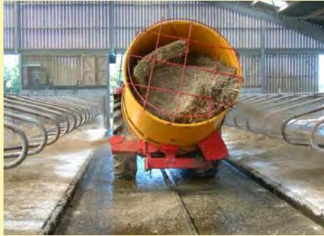
**T4040 AND T5050** handle 4, and 5' diameter round bales. Discharge from either side or both sides. Lower left and upper right discharge chutes spread material evenly into stalls.
