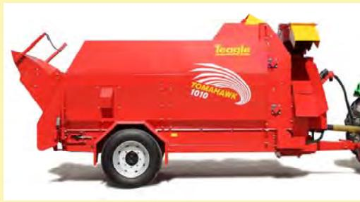
**MODEL 1010** will handle up to three 6' diameter round bales or two 8' long rectangular bales in one load.
