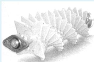
Aggressive 56 knife rotor with spiral design assures an even power curve for uniform continuous cutting less horsepower. Reversible knife plates slide easily onto 1 1/4" hex shaft.
