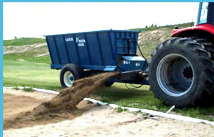
**LUCKNOW'S MATERIAL HANDLER** can be used to spread/discharge materials up to 16' away. 7 cubic yard capacity.
