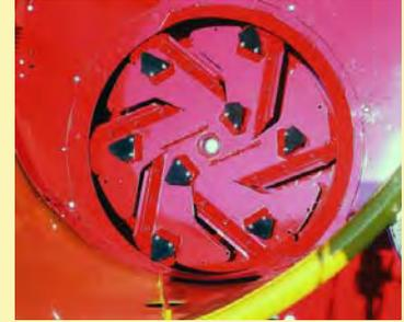
Heavy duty silage rotor handles all types of hay and straw. Machines can be run at 540 RPM or 1000 RPM when greater distance is needed.
