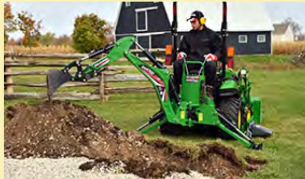
**Model GE605** for 18-28 HP tractors or mini skid steers. Digging depth of 6' 4" and a 100" reach.
