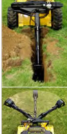
**"BIG ARM" SKID STEER BACKHOE** with up to 12' reach height and 110 degree swivel.
