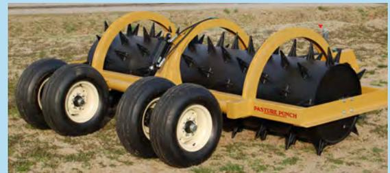
**PASTURE PUNCH AERATORS** in 6', 8', 10 and 12' widths. Relieves compaction, promotes air and water movement, relieves root bound plants, helps activate fertilizer. (Interchange spiked rollers with smooth rollers for dual purpose)
