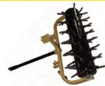
**4', 5', AND 6' SPIKE AND PLUG AERATORS** can be used as 3 point or pull type.
