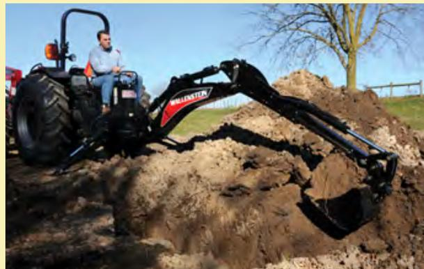
**Model 920XT** with foot pedal controlled hydraulically extendable dipper stick adds 24" of digging depth.
