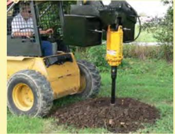
Weighted frames give added down pressure for fast digging in tough conditions. Weighted frames of 1400#, 1900#, and 2400# are available
