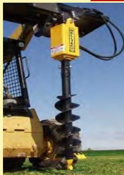
Belltec **NC-Series** hydraulic auger drives are available in three models for systems operating between 6 and 30 GPM and 2000 to 3000 PSI. NC-Series auger drives are designed with a planetary gearbox to eliminate chain and sprocket reductions found on drives in this class and price range.
