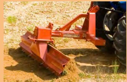
**LAND PLANES** - Ideal for gravel road reconditioning, driveway grading, pot hole filling, and general land leveling and grading. All land planes perform with much more efficiency than large motorized graders and are cost effective for small grading jobs.
